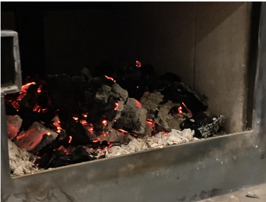
iv. Picture after test fuel load adjustment (6:04:00 run time)
