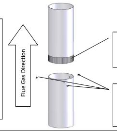
Crimped or male end of single wall chimney connector must face down.
