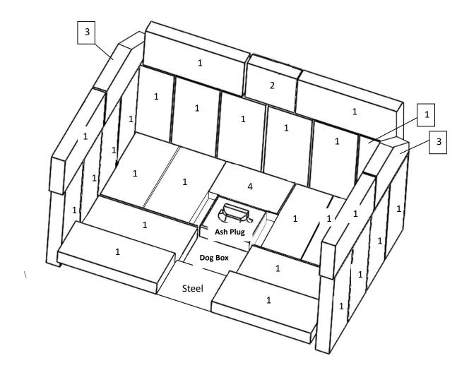
NOTE: The bricks on the sides and rear will need to be installed after delivery
