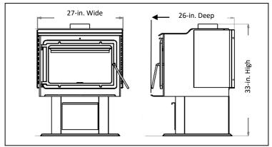
Dimensions are approximate. Be sure to locate your stove in the installation area before installing pipe, etc.
