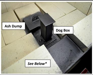
\*DAILY --Inspect the firebox for ash accumulation; remove excess ash and follow instructions in your owner's manual regarding disposal. Ash should not be allowed to accumulate in the stove to the point that it covers the dog box hole. The ash dump plug in the firebox may be removed and ashes raked into the ash pan below for temporary storage. Remember to replace the ash dump plug.
